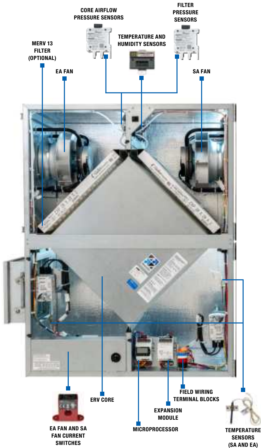
FIGURE 1.5.0 SENSOR LOCATIONS IN ERV UNITS, HE10INV SHOWN
