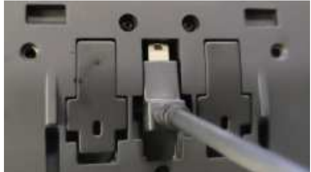
Figure 3-7. Inserting USB Cable into USB Port
