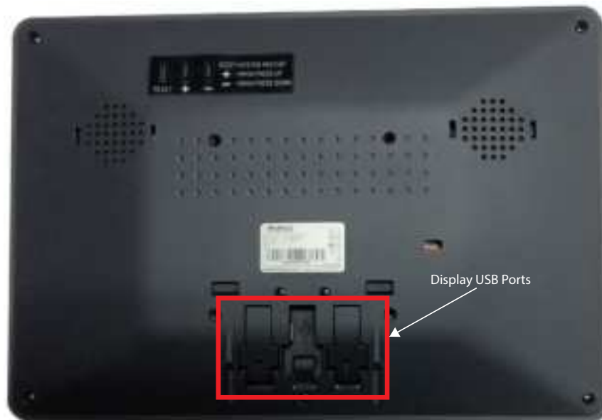
Figure 3-5. Display USB Port Location
