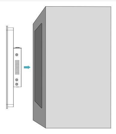
4. Align the screw holes (non-threaded) of the snaps with the snap mounting holes on the device side.
