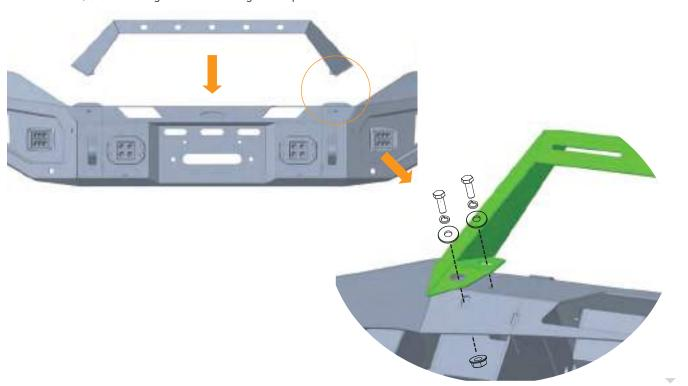
Assemble the license plate brackets using the (2)M6x16mm button bolts, (2) M6x12x1mm flat washers, (2) M6x12x1.3mm nylon round spacer, (2) M6 nylon lock nuts.
