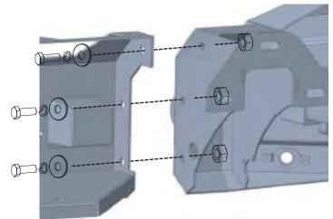
Install the bull bar to the main body using the (4) M8x20mm hex bolts, (4) D8 lock washers, (4) M8x20x2mm flat washers, (2) M8 flange lock nuts. Tighten up all bolts.
