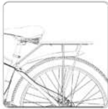
11. Press the rear fender down and install the rear rack.
