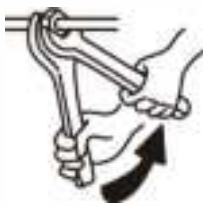
Fig. 4.2 Tightening Work of Flare Nut
