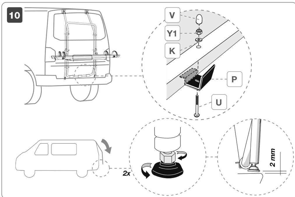
**EN** To fix the lower brackets, it is necessary to pull down the structure. Make sure that the fastening of the Carry-Bike is steady.
