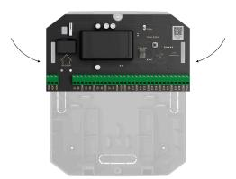
**4.** Install a 12 V= backup battery at the special fixation racks in the casing. Note that third-party power supply units cannot be connected to the terminals.
