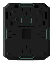
2. Secure the casing on the vertical surface at the selected installation location with the bundled screws using all fixation points. One of them is in the perforated part above the tamper — it is required for tamper triggering in case of any attempt to detach the MultiTransmitter casing.
