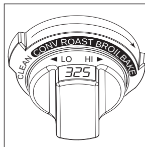
Figure 3-31. Turn Control Knob Bezel Clockwise to Dark Area Marked ROAST
