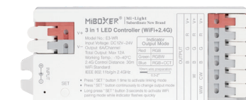
E3-WR 3 in 1 LED Controller (RGB / RGBW / RGB+CCT)
