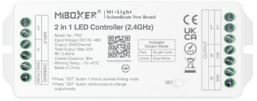
PR2 2 in 1 LED Controller (Single Color / Dual White)
