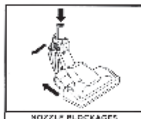
NOZZLE BLOCKAGES Detach the hose. Pull the bottom of the neck out of the connecting, and release the top of the hose by squeezing the tabs together. Check the hose and the openings for blockages.
