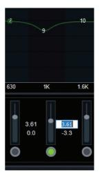
**Gain**: Gain can be adjusted by using the up/down arrows when the band's EQ dot is highlighted. You can also click into the gain or Q rows of any band and adjust with the up/down arrows. You can move from one band to the next with the right/Left keyboard arrows.
