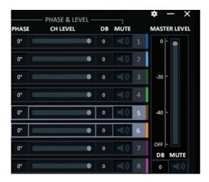
There are a number of systems for checking System Phase. If the systems speakers are not all in phase there will be issues you can not fix by tuning. You can see the section on System Phasing to see one method of Phase checking. The MUTE buttons allow you to turn off any speakers that you do not want to hear while you are tuning other speakers.
