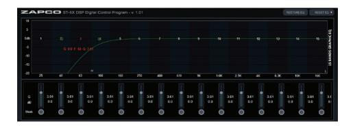
Here are 15 bands of parametric equalization for each output channel and you can vary Frequency, Gain, and Q (the shape of the adjustment) for each band in several ways.
