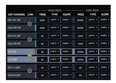
You can select a channel to tune by clicking on the desired speaker in the car diagram/Delay section or by clicking on its box in the DSP Channel column. You can pick channels on at a time or you can pick them by pair. Double clicking the dot between a pair of channels links that pair. Similarly, if one channel is already chosen and active, then clicking on the dot will pair them.
