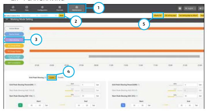
**Peak Shaving:** The user can define a timeframe of when the system will compensate for the power pulled from the grid for loads during peak demand times to avoid higher electricity rates.
