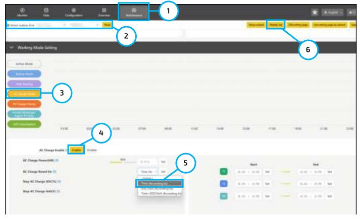
AC Charge Mode: Allows the grid to both charge batteries and power loads.
