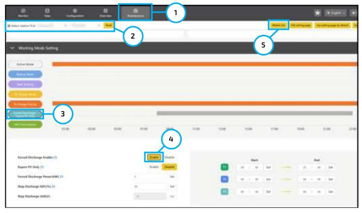
Forced Discharge: Forced discharge prioritizes battery power for powering loads and grid sell back.
