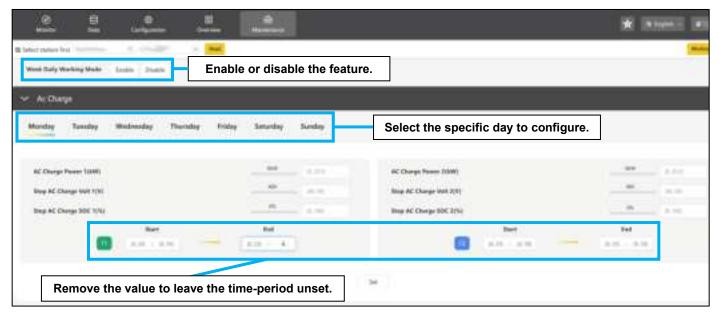
When the weekly setting is enabled, the priorities for the functions are:
