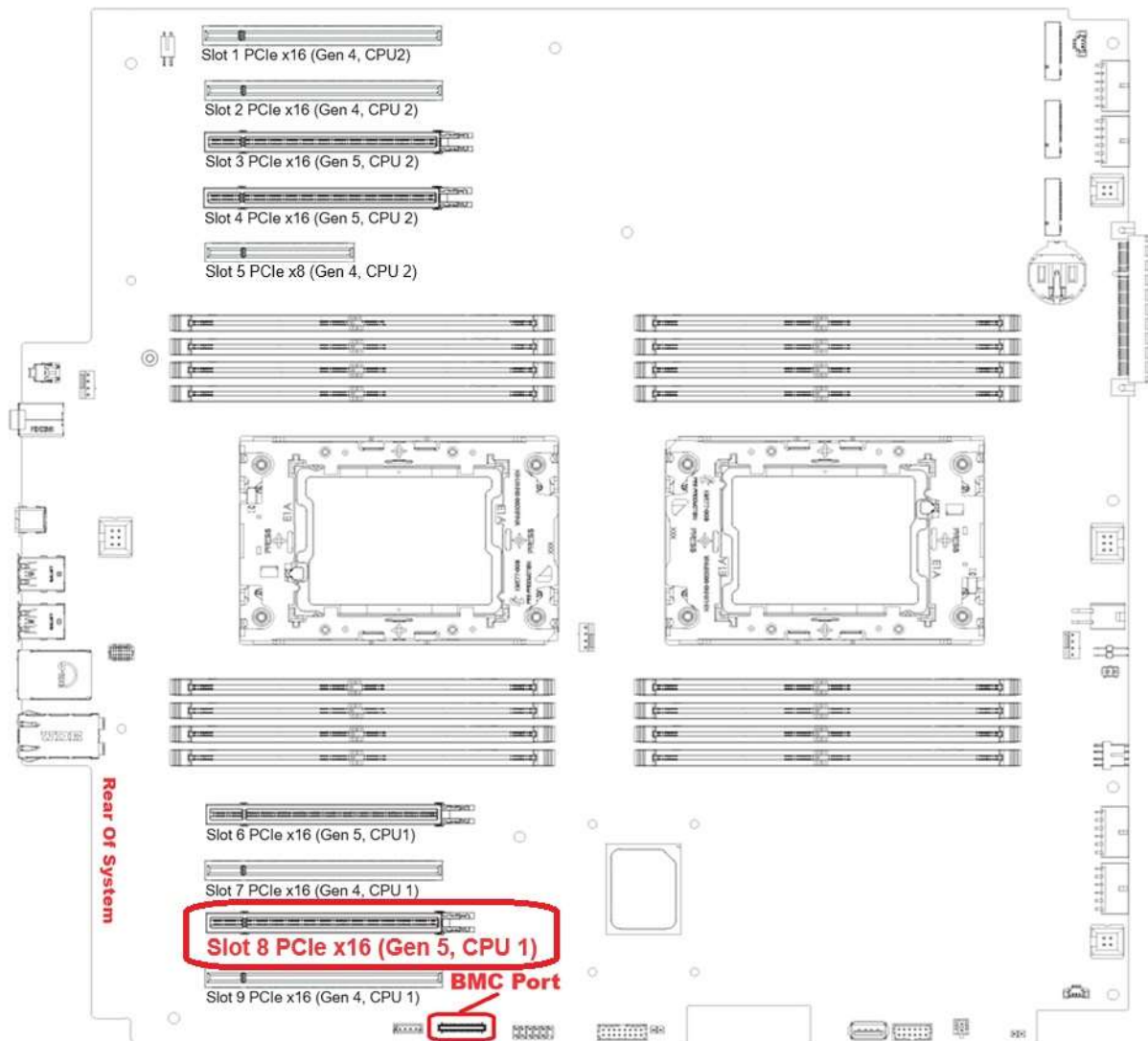
Figure 9, PX Motherboard BMC Port Location and BMC designated PCIe Slot 5
