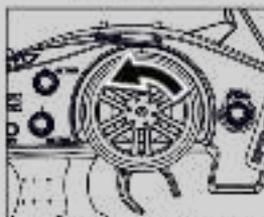
Go to Full Left Steering on the transmitter. Blue LED on ESC will flash once and wheels will turn to the left.
