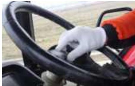
c) Pull out the steering wheel forcefully. If it is difficult to remove, it is necessary to strike the spline shaft to loosen it with a hammer and to be careful to avoid the steering wheel damage, or use of high quality puller tool to avoid damage on original steering wheel and shaft
