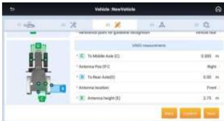
**To Middle Axle(C):** If the receiver is not mounted on the central axis, measure the distance from the receiver to the central axis. If it is on the central axis, enter 0. In reality it is always better enter 0 and do the rest in assembly error calibration.
