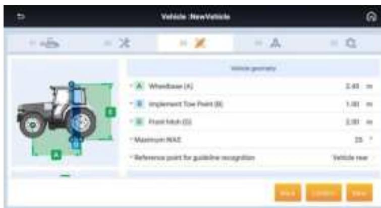
**Wheelbase(A):** Measure the distance between front wheel rotation axis and rear wheel rotation axis. Note that the tape measure needs to be parallel to the ground.
