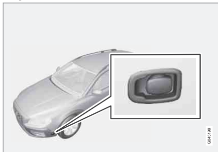
Electrical input to the engine block heater.
