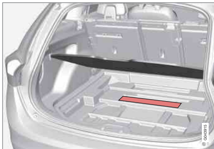
Storage space, safety net cassettes.
