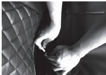
Connect the two air plug and the wire firmly.
