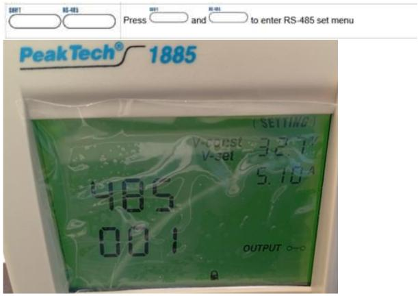
a. When the device address of RS-485 is between 001 and 009, we must regard the <address> as "01"
