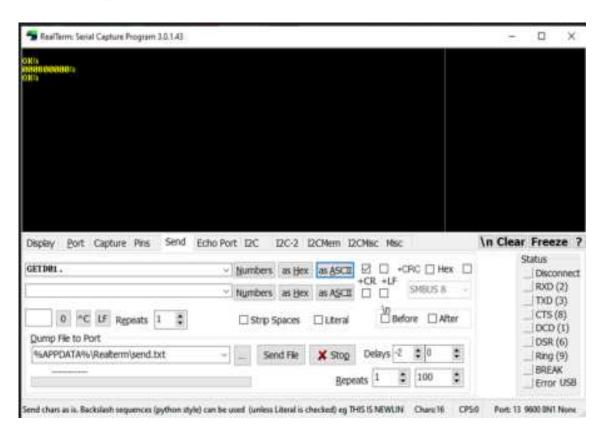
b. When the device address of RS-485 is greater than 9: We must convert it from Decimal to Hexadecimal and then to ASCI Code. For example, for an address "010", we must regard the <address> as "010" or "0A" or "0:".
