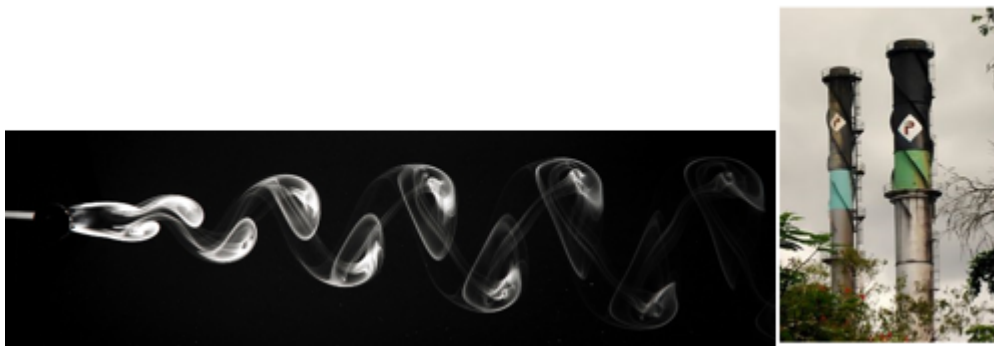
Figure 30: Vortex Shedding Formation Downstream of a Cylinder (left) and Chimney with Spirals (right)
