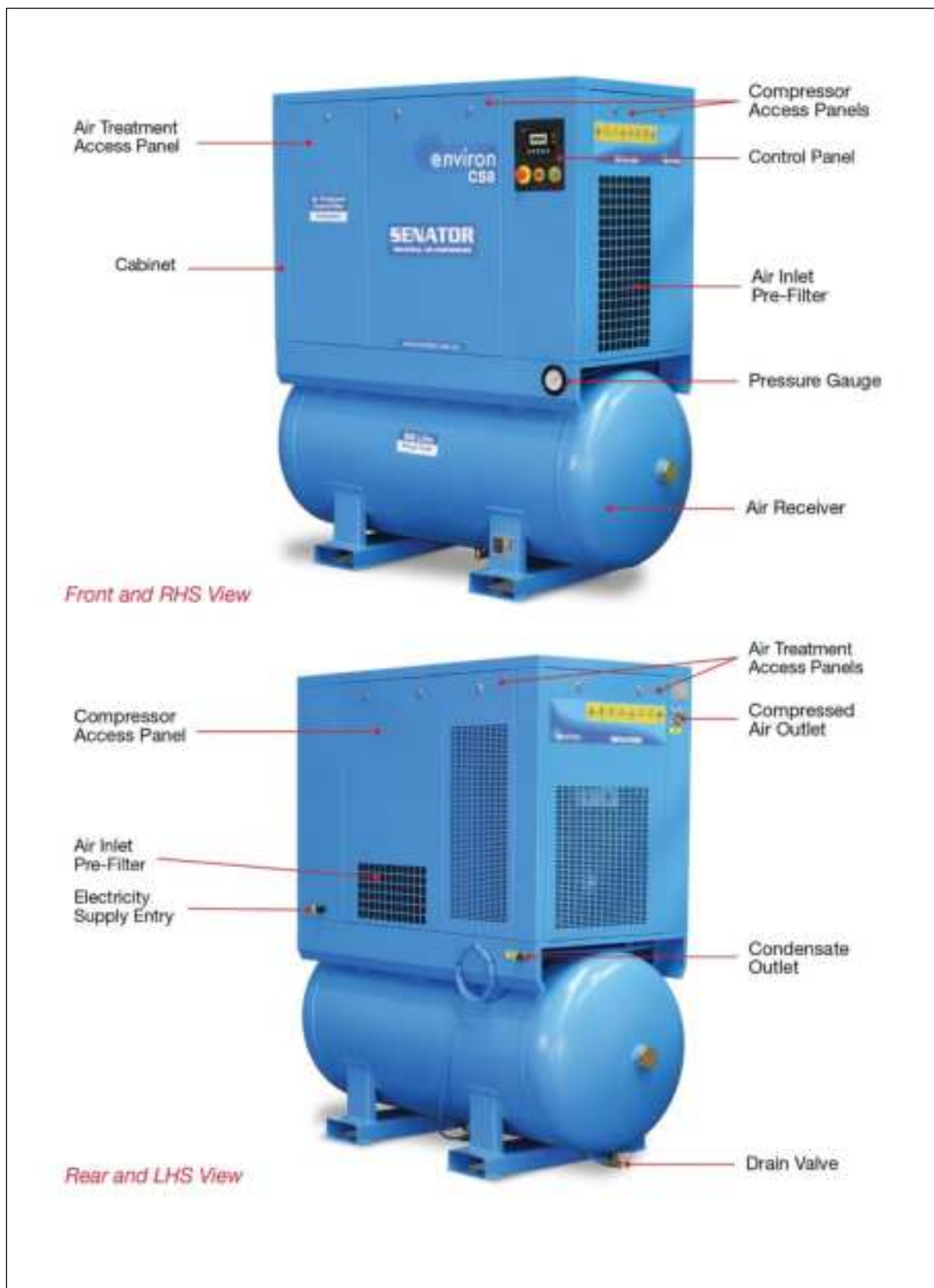
Figure 3-2 External Features of CS Series Air Compressor Set
