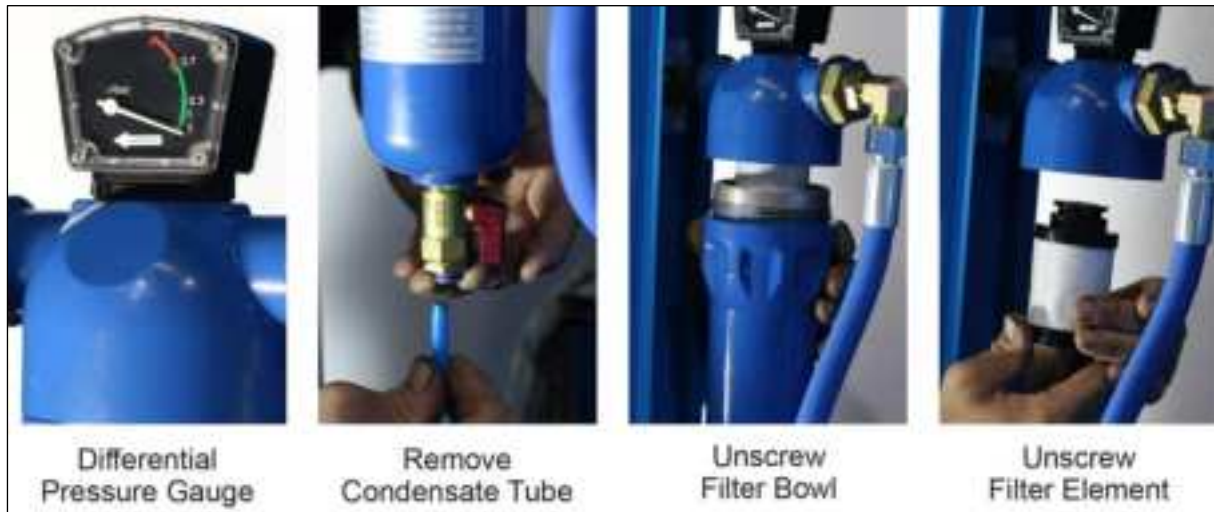
Figure 6-4 Compressed Air Filter Replacement
