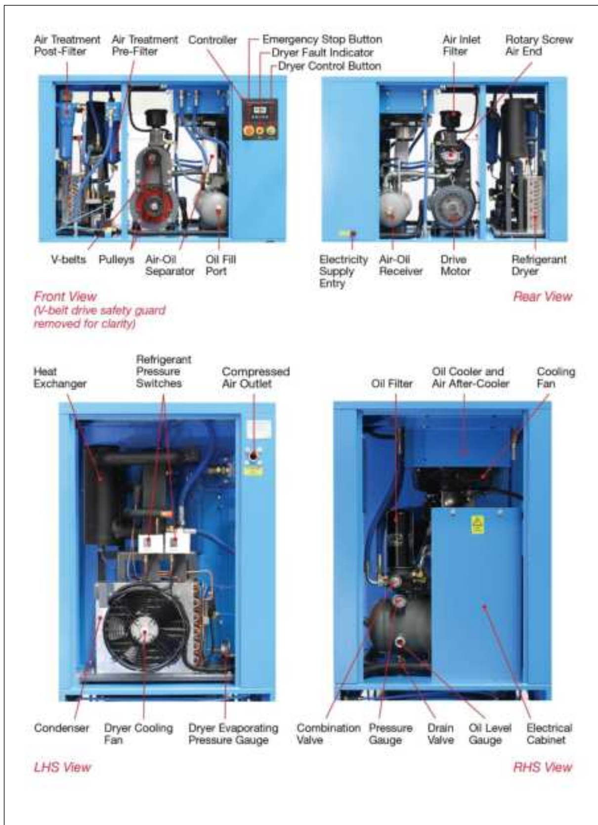
Figure 3-3 Internal Features of CS Series Air Compressor Set
