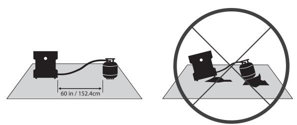
Set the fire pit and LP tank on stable, level ground. Ensure 60 inches (152.4cm) distance between LP Tank and fire pit. Locate the gas hose in a safe place away from walking areas to avoid tripping on the gas hose.
