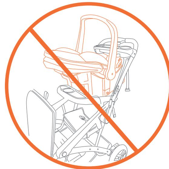
**DO NOT** use a single car seat in the rear seat position. **DO NOT** use the rear seat without fabric installation.
