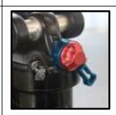
**Handlebar-operated roll lock** with trike stopped and driverless to keep bike stable without a kickstand.
