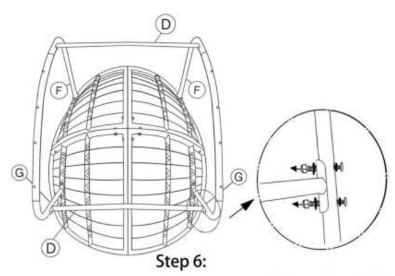
Aligning two screw holes on (D) and (G), Using (N) to connect and fix together Install (D) first and (E) last!!
