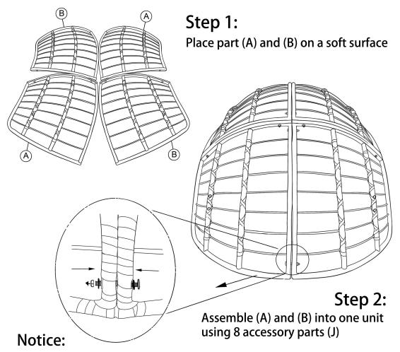
1-Please don't tighten all screws completely at beginning!! 2-Fully tighten after completing the seat frame!!
