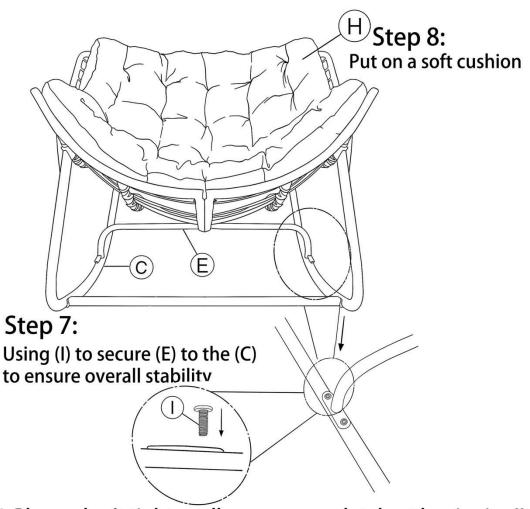
1-Please don't tighten all screws completely at beginning!! 2-Fully tighten after completing the chair legs!!
