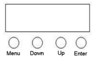
The LCD system includes Menu, Down, Up, and Enter buttons. Press "Menu" to enter the menu or to go back from a sub-menu. Use "Up"/"Down" to navigate through the choices, and use "Enter" to save your choices.
