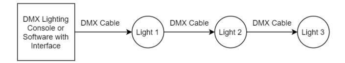
**32 Fixture Rule** – DMX only allows you to connect up to 32 fixtures in a single daisy chain for signal strength. Sometimes, depending on the fixtures and cable length, this number is less (or more).
