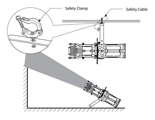
Never stand directly below the device when mounting, removing, or servicing the fixture.
