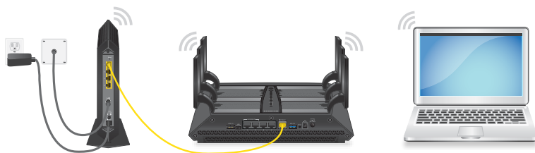
Figure 7. Connect the cable modem to a router
