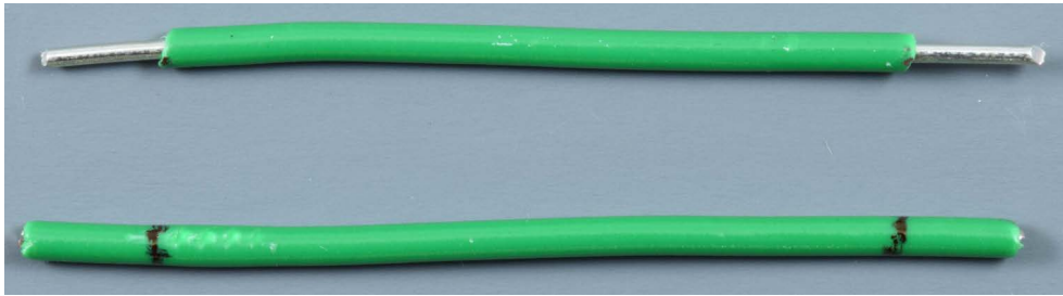
Figure 9. One wire marked and another one stripped. The insulation left should be 3 cm long.
