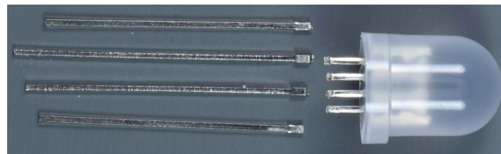
Figure 6. The leads of RGB LED WS2812D-F8 cut just above the widening.
