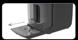
Pull out the Drip Tray (8) from the Main Unit (23) (if needed).
