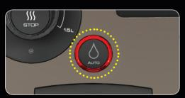
Place a vessel underneath the Dispense Nozzles (6) and press the Dispense Button (5) to reset the system. This takes approx. 25 seconds. Any water dispensed during resetting should be discarded.
