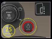
Press the Dispense Button to reset the system. Any remaining water will be dispensed from the system into the vessel below. This takes
