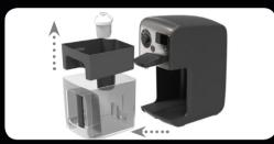
Remove the Water Tank (7) from the Main Unit (23). Remove the BRITA MAXTRA Cartridge (19) and BRITA Hopper (21) from the Water Tank.
