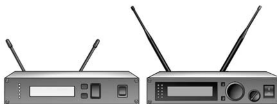
1/4 wave and 1/2 wave antennas: UHF range
