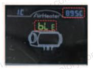
**2.Connect to the mobile phone via Bluetooth :** Click on the Bluetooth symbol in the upper right corner, find the corresponding local Bluetooth number : BYD + MAC address of the Bluetooth device + 4 digits from the controller(Refer to the picture above), then click on the Bluetooth number to connect;
