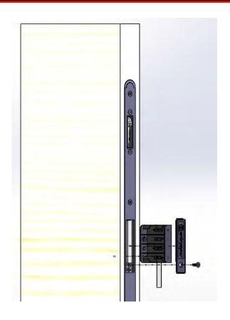
Remove screw, battery door and empty battery pack.
