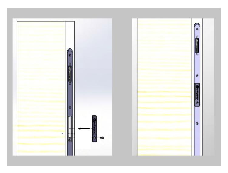
Replace battery door and screw. Ensure the pull tab for battery pack is installed such that it does not interfere with the screw installation.
