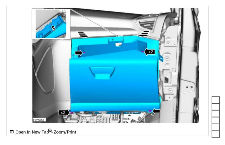
10. Disconnect the BCM electrical connectors and remove the BCM.
