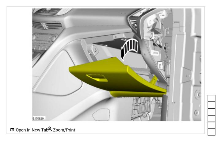
9. Remove the screws and the glove compartment.
