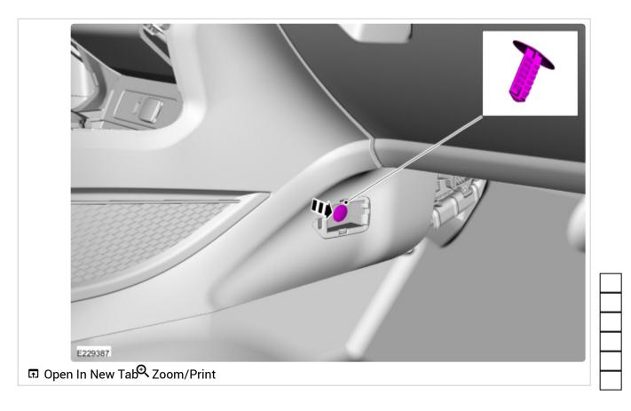
7. Remove the bolt, release the clips and remove the RH floor console finish panel. *Torque*: 22 lb.in (2.5 Nm)
