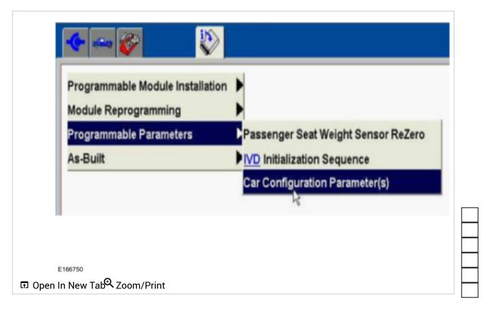
6. **NOTE:** If a diagnostic scan tool is connected to the internet, it automatically obtains As-Built data. If a diagnostic scan tool is not connected to the internet, obtain the As-Built data from PTS OASIS. Download the As-Built data to the scan tool or other storage device, such as a flash drive, following the on-screen instructions.
