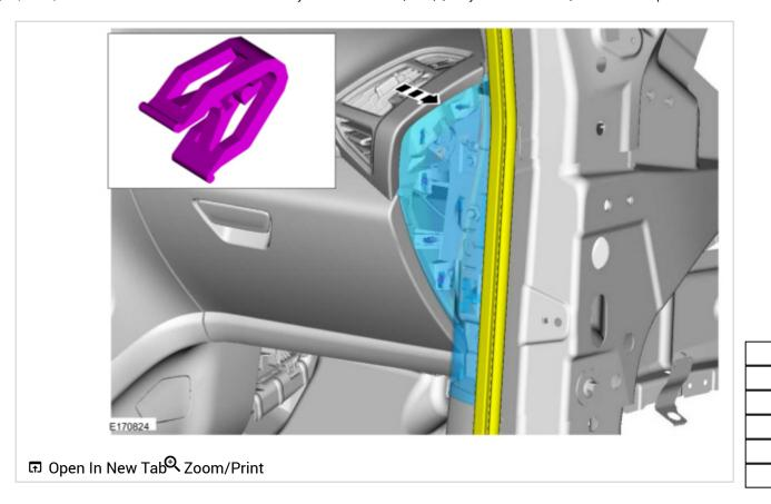
4. Detach the clips and remove the RH instrument panel lower finish panel.
