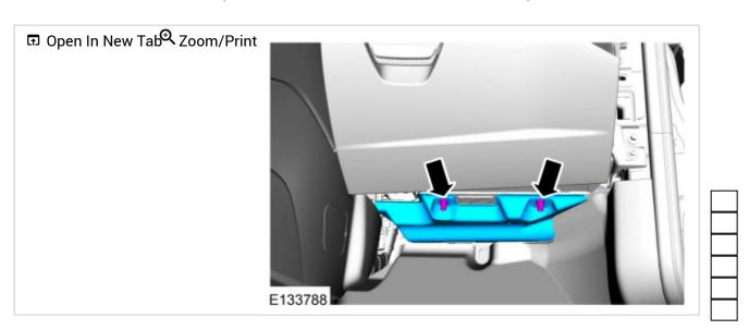
3. Position the front door weather-strip aside and remove the instrument side trim panel.
