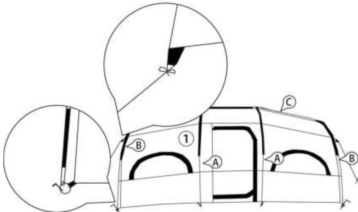
**EN**\_4. Cover the outer cover and place it in the corresponding position with a D-bar
