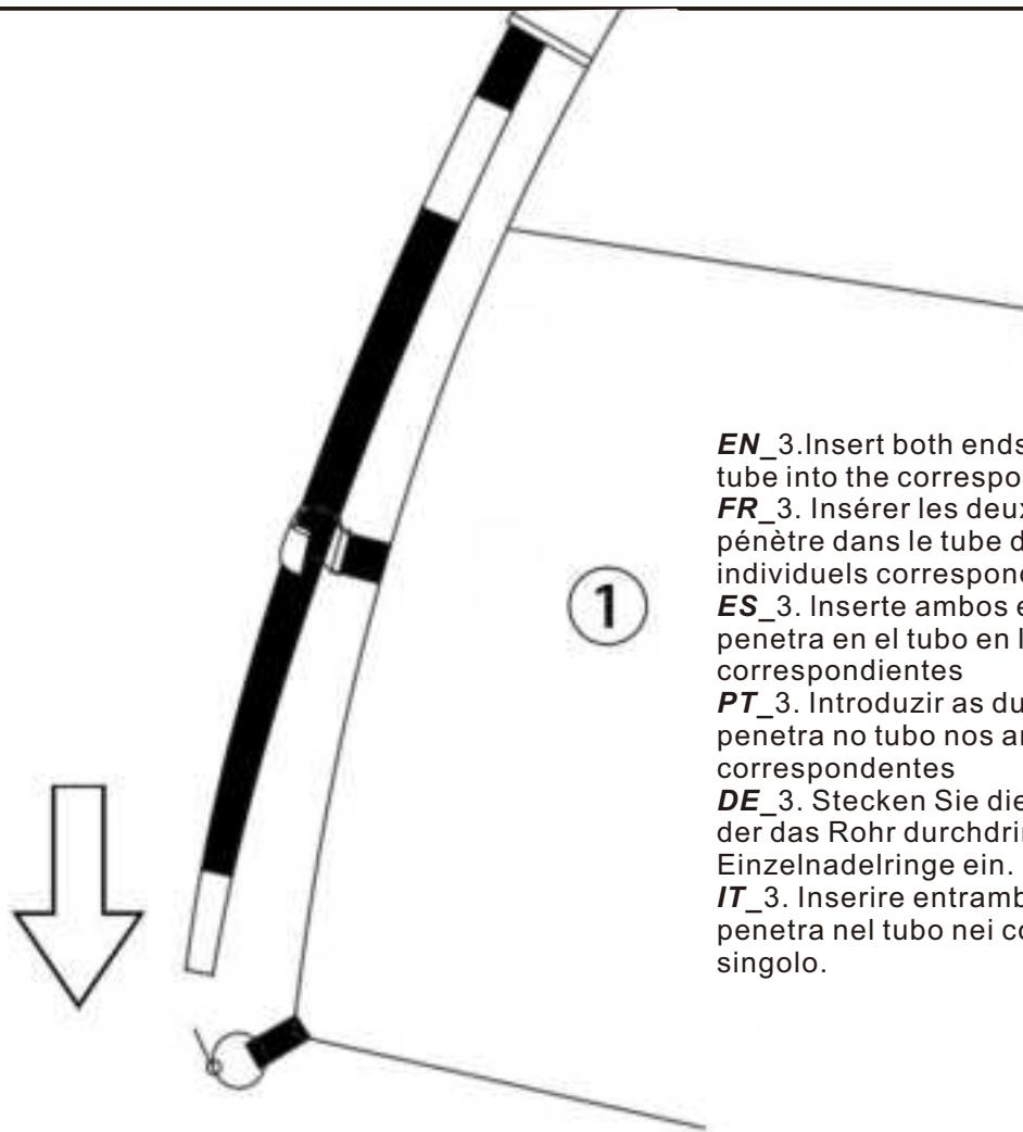
**EN**\_3.Insert both ends of the rod that penetrates the tube into the corresponding single needle rings
