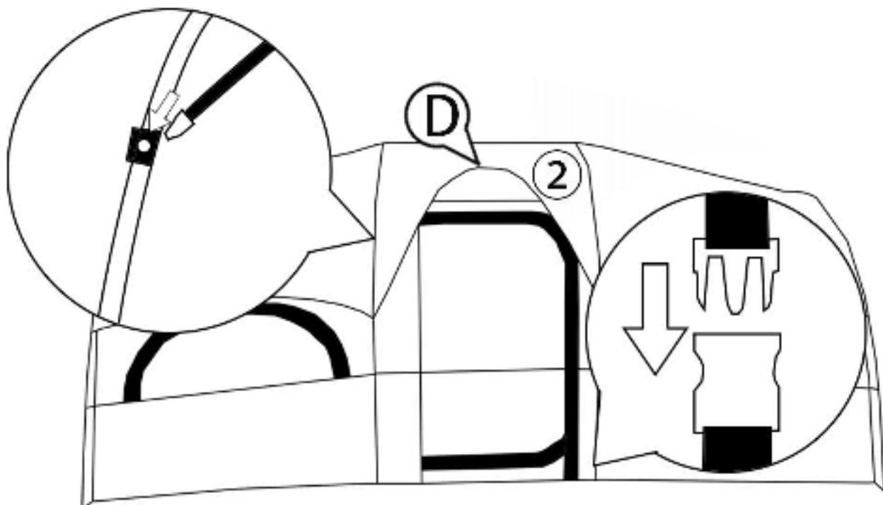
**EN**\_6. Put the outer cover of 2 onto the inner tent and secure it with the corresponding backpack buckle at the corner. Fix the D-pole as shown in the diagram
