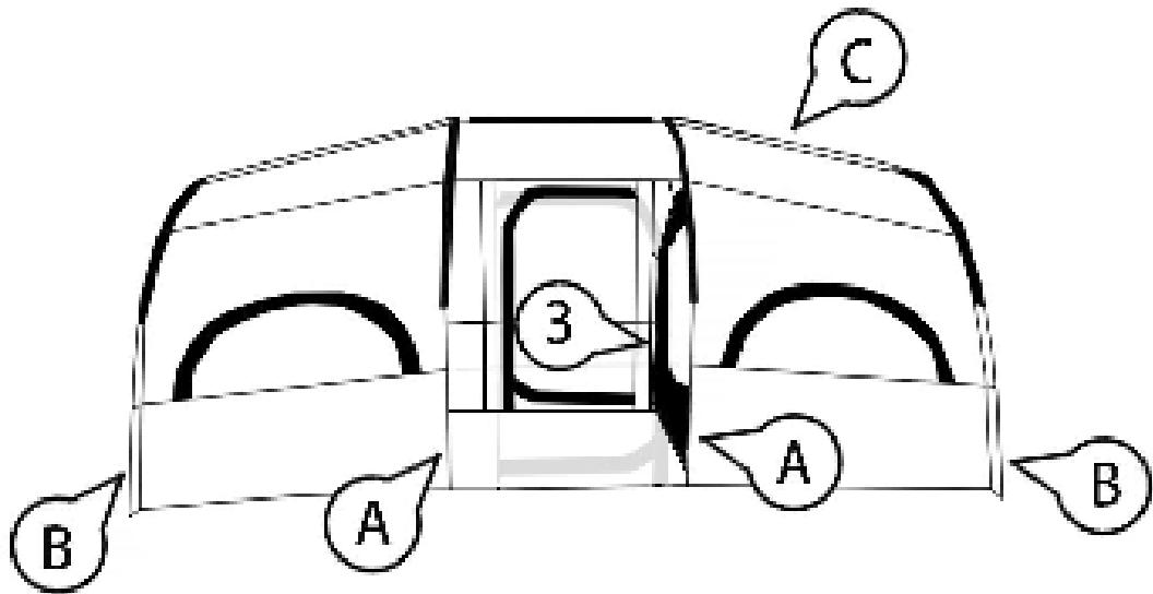
**EN**\_2.Thread the A/B/C rod into the pipe as shown in the diagram and clip it into the corresponding pipe sleeve
