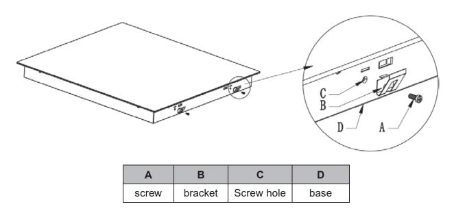
Adjust the bracket position to suit for different work surface's thickness.
