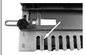
Line up the inside edge of the left horizontal stop with the line you just drew on the template. Use a set square to ensure the stop is square to the jig.
