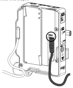
Attach to camera using ARCA interface. Adjust vertical position and lock thumbscrew. If additional tightening is required, pull out thumbscrew handle to ratchet.
