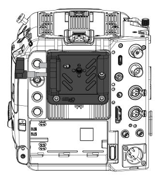
For Remote Start / Stop function (R/S), install 2.5mm TRS Cable into DB-10 REMOTE port.
