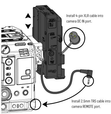
When using wide batteries, adjust battey plate position to expose power outputs.
