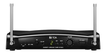
The WT-5810 is a PLL-synthesizer controlled double superhetrodyne diversity tuner designed to be used with a UHF wireless system. It employs a compander noise reduction circuit to minimize the influence of ambient RF noise.
