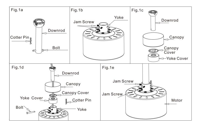
WARNING: Do not loosen the lower jam screws under any circumstances.
