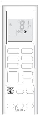
The air direction and flow rate are adjusted so that the air will not blow directly at people in the room.
