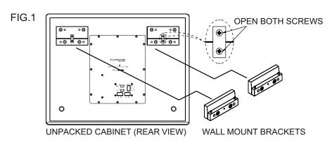
Next, drill holes on the wall for the screws supplied, as per the following diagram, where you want to mount the SSW 2020. Please see Fig. 2 below Now fit the wall mounting brackets to the wall with the help of the screws supplied. Please see Fig. 3 below
