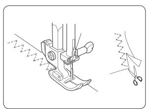
This stitch is used to finish a raw edge on synthetics and other fabrics that tend to pucker. Place the fabric to leave a 5/8" (1.6 cm) allowance.
