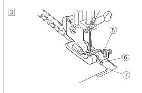
3 Turn the screw to align the guide on the foot with the folded edge so that the needle just pierces the fold.
