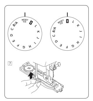
Now, simply step on the foot control to sew an identical buttonhole.
