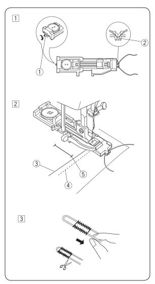
With the buttonhole foot raised, hook the filler cord on the spur at the back of the foot.
