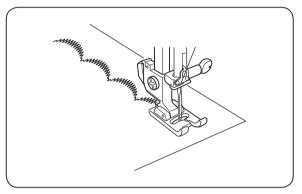
Determine the appropriate stitch density by test sewing.
