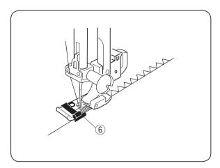
Overcasting is used to prevent fabrics from raveling at raw edges. It can be used to finish a hem edge.
