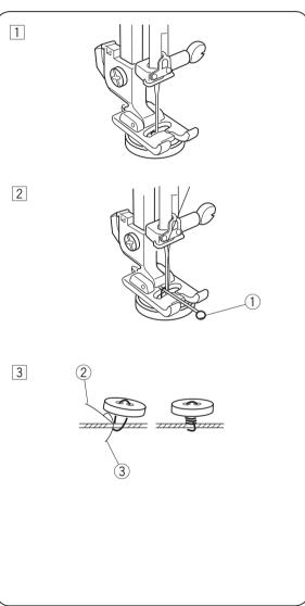
1 Unthread the needle. Adjust the stitch width to match it with the span of the holes in the button. Turn the handwheel to check if the needle enters into each hole in the button. Lower the foot to hold the button in place. The holes in the button should align with the slot of the foot.
