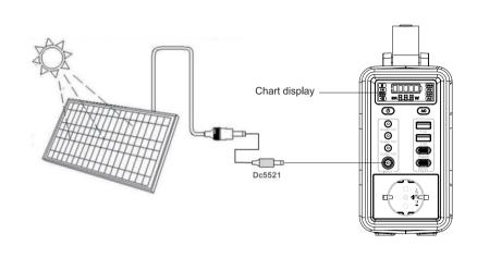
A.Place your solar panel where it will get as much strong direct sunlight as possible. B.Connect the output port of the solar panel with the input port of the product to start charging. You will know the product is being charged when the LCD display indicators blink. The product is fully charged when all battery indicators stop blinking and remain solid.
