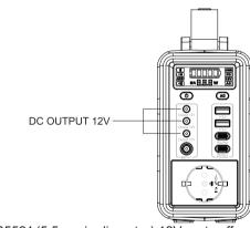
A. These three DC5521 (5.5mm in diameter) 12V ports offer max 10A output current and automatically distributing max current according to the external connected devices to ensure shortest charging time
