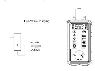
Plug the original adapter into the machine's AC input port and you will see the battery indicators on the screen blink.
