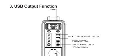
When two USB-A and the USB-C port charging simultaneously, the three ports can only output 5V/5.6A in total.
