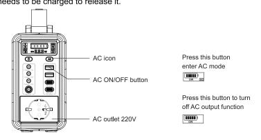
A. Press the power button to enter AC mode. Plug the power cable of AC appliance B. Make sure the power of the connected AC appliance is less than 200W.
