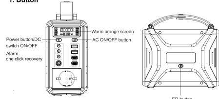
A. Long press the power button for 3 secs to turn the machine on. Press this button again to turn on DC function. B. Press the AC button to turn on the AC function. C. Long press the AC button to turn off the sound. D. Press the POWER/DC button and AC button simultaneously to switch the frequency of the machine;
