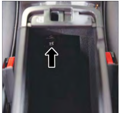
Center Console Power Outlet
