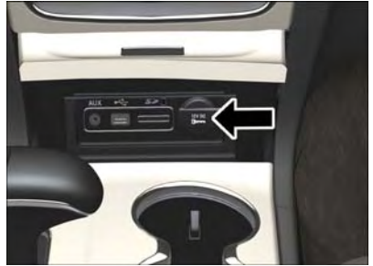
Front Power Outlet
