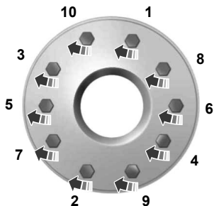
10-lug nut torque sequence.
