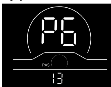
Fig. 7-6 Current Limit Setting Interface
