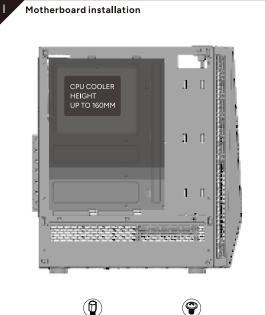
According to the motherboard type (ATX/M-ATX/ITX), the copper pillars may need to be re-arranged manually according to the fixing locations specific to your motherboard CPU Height limit: 160mm
