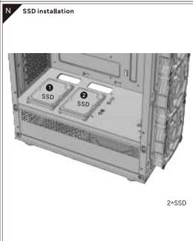
Align the SSD holes and fix them with screws.
