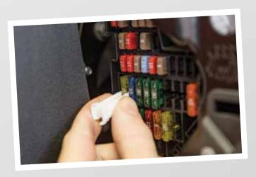
Remove the fuse for the "Horn" circuit from the fuse box in order to cut the power supply of the acoustic signaling units for the duration of the electric connection.
